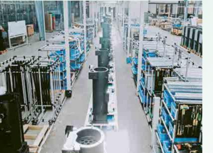
With the setup of a lighthouse area for the assembly of the 20 – 32 kW Nano-Pellet boiler according to lean principles, it was possible to sketch out significantly higher area productivity. The insights gained were used to design the fine planning of the work systems and implement logistics processes in the new hall.
